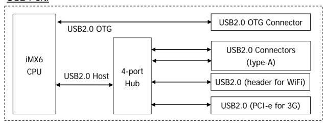
NOTE: The USB 2.0 OTG can be used in host mode or device mode. If you would like to use it in host mode, a separate OTG-to-host cable is required.
