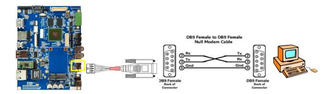
UART1 is dedicated as the debug/console port. UART1 default settings are **Baud Rate 115200**, **8 data bits**, **no parity**, **1 stop bit and no flow control**.
