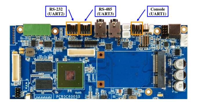
One 2x4 box header to DB9 cable is included. See **Appendix A** for the detailed info on the cable pin assignment.
