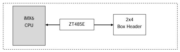
ZT485E: RS485 transceiver. RS485 works in half duplex mode.
